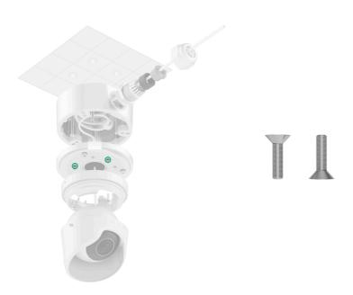
**3.** Place the camera enclosure in the holder, ensuring that the camera lens faces the protected area. Secure it in place by tightening the two screws in the holder using the bundled hexagon key (Ø 2 mm).
