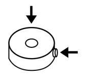
Two options for cable gland installation: at the top or at the side
