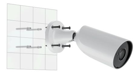
**8.** Loosen the screw on the swivel mounting bracket to adjust the camera tilt and rotation position.
