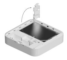
**4.** Install the hard drive in the NVR enclosure so that the connectors match.
