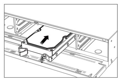
Figure 1-7 Insert HDD
