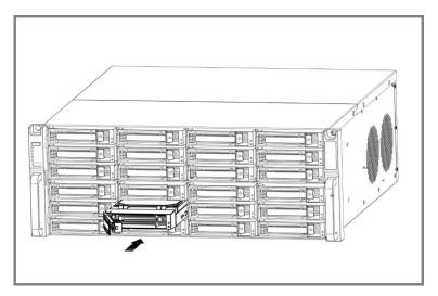
Figure 1-9 Push HDD Case into Slot
