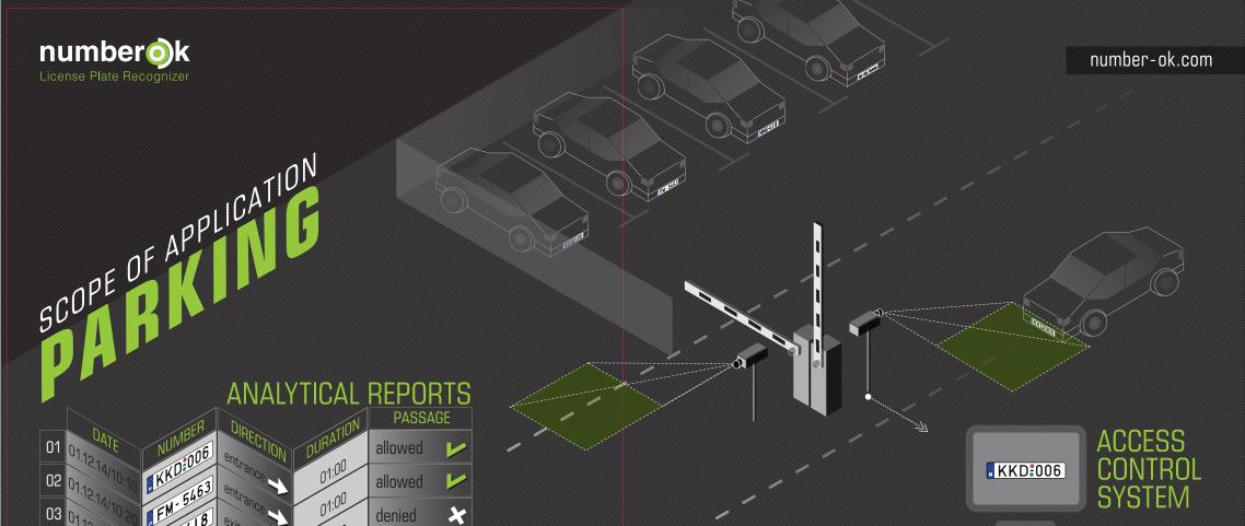
The main objective of NumberOK installed at the parking is the counting of the vehicles and identification of time they spent at the parking lot.
