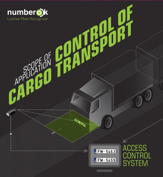
Many transportation providers have faced the problem of capturing license plate numbers of cargo transport, as the number plate of the car and the trailer is different.
